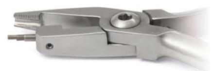
Loop forming plier Tweed style For round and rectangular wires. Replaceable cylindrical beak with three sizes: 0.045" (1.14 mm); 0.060" (1.52 mm); 0.075" (1.90 mm)
