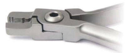
Lingual arch plier To form double or triple back bends in wires of 0.030" (0.76 mm); 0.036" (0.91 mm)
