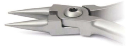
Rounded jaw wire bending pliers, long beak To bend wires up to 0.020" (0.51 mm)
